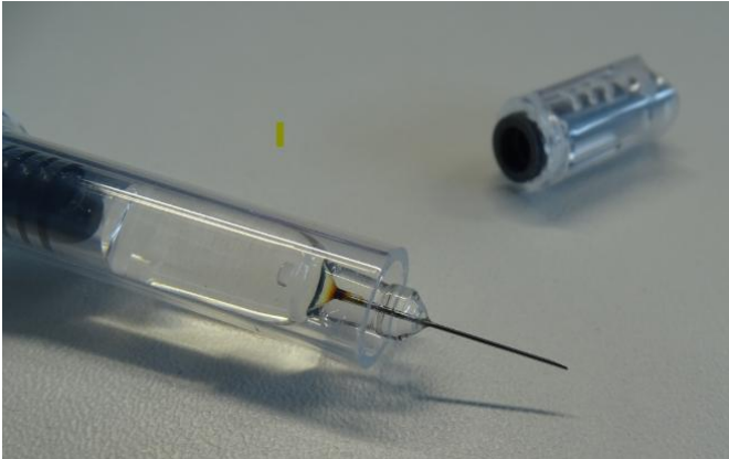
Figure 1: Example of syringe with discolouration at the base of the needle
